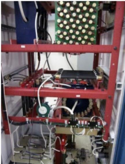
**Figure 2.** High Voltage Cabinet. Clockwise from top left: Switch Plate; Snubber Circuit; Grid and Screen Plates; Filter Capacitor; Storage Capacitor.
