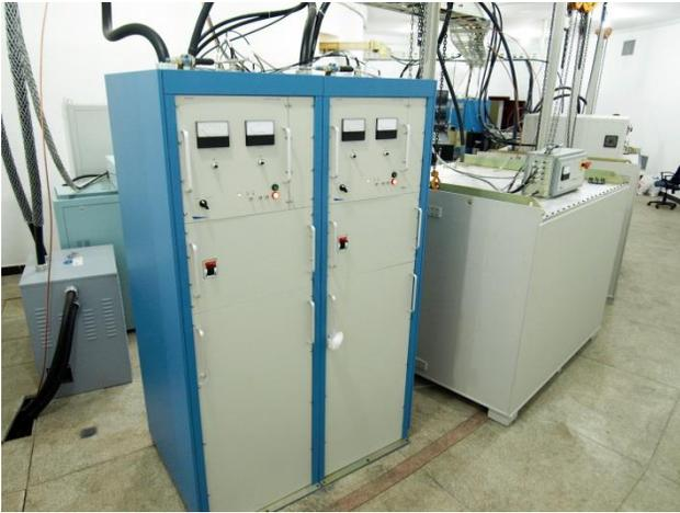
**Figure 2. Installation of the 2 MW klystron transmitter. View shows DTI's high voltage power supplies (left) and capacitor tank (right).**
