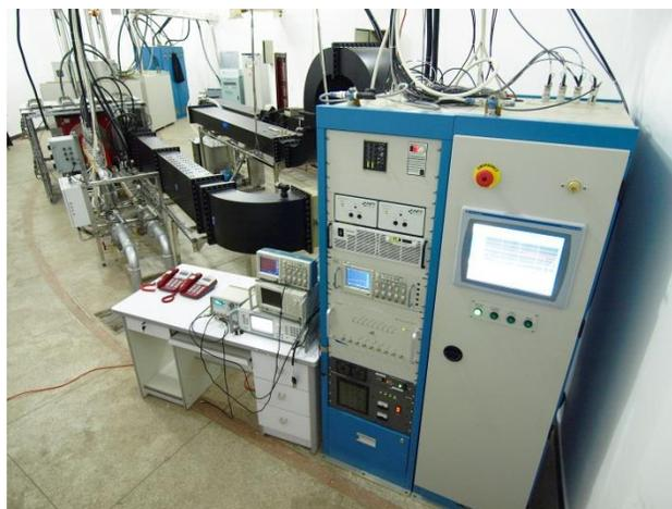
**Figure 7. Installation of DTI’s transmitter for a 2MW, 500 MHz klystron. Note the blue high voltage power supplies and light gray modulator tank in the far back, klystron, water manifold and black waveguide in the center and RF driver, microwave control unit, PLC and graphic interphase unit in the foreground.**
