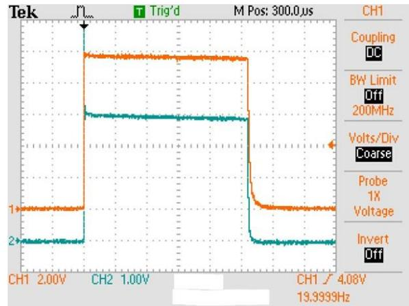
**Figure 4. Scope shot of 100 kV pulse into resistive load, 520 µsec Ch1 V<sub>k</sub> 99 kV (10 kV/div); Ch2 I<sub>k</sub> 41A (10A/div).**
