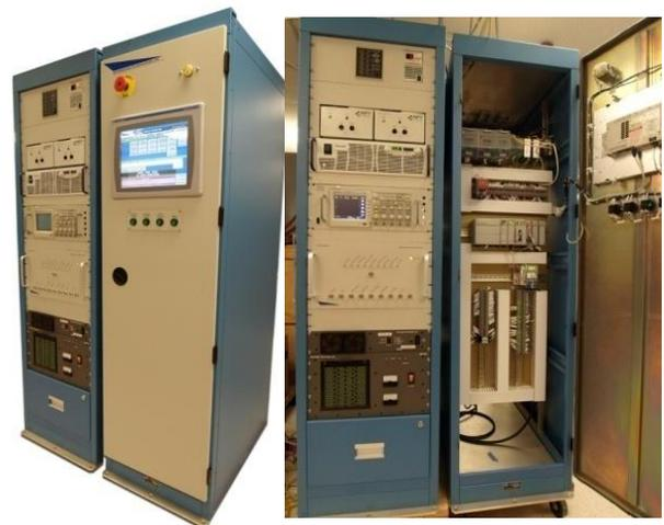
**Figure 5. Controls racks for the 2 MW klystron transmitter.**
