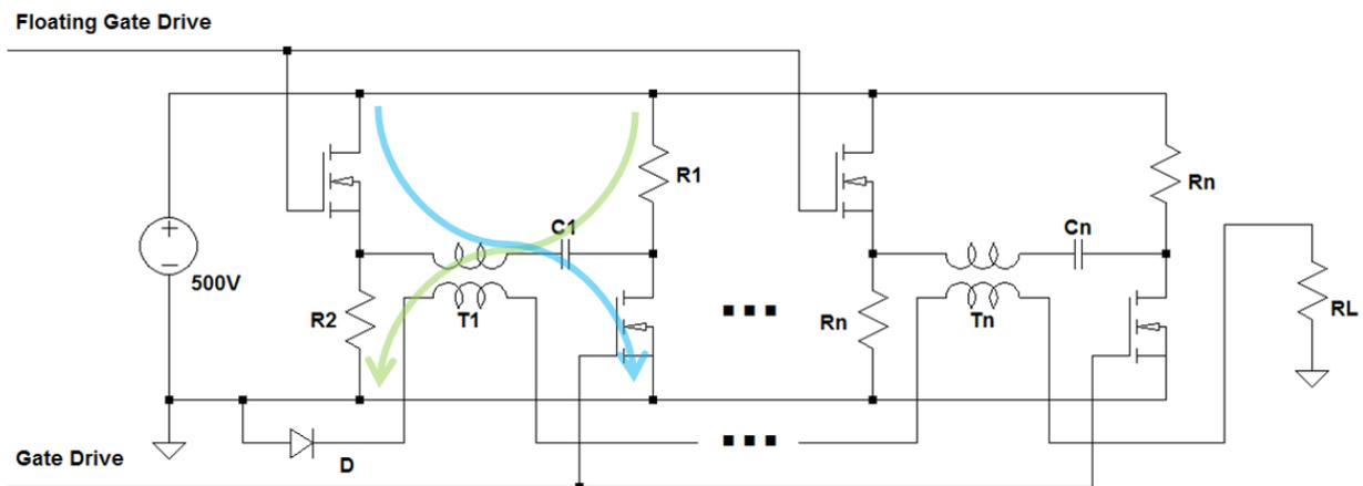
Fig. 2. Electrical schematic of two stages showing main pulse current path in blue and charging current path in green. The floating gate drive is referenced to the source leads of the "flying" transistors. For clarity, snubbers and clamp diodes are not shown. Diode D isolates the transformer core reset voltage from the load.
