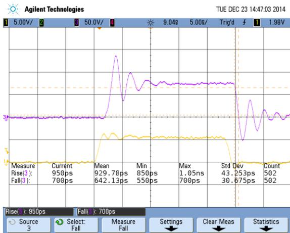
Fig. 3. Performance of the gate driver circuit with GaN transistors in a test board, operating from 75 V into 1.5  $\Omega$  and 3.3 nF, or 50 A peak. Note the 950 ps rise time, 700 ps fall time, and 1.5 ns group delay.
