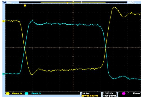
Fig. 4. Bipolar operation of two kicker boards into 50  $\Omega$  each side, 5.8 kV (+) and (-), 5 ns rise, 6 ns fall, 30 ns flattop. Due to the simple transformer arrangement of the output, setting up the pulser for bipolar or unipolar operation as simple as moving bolts.
