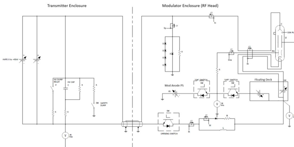
**Figure 1. Simplified transmitter schematic.**
