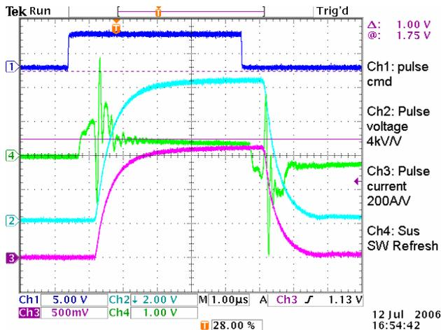
Figure 4. Sample pulse from the PEF system shown in Figure 1, at 34 kV, 320 A, 4  $\mu$ S flattop.
