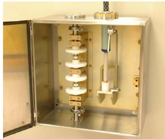
*Figure 3. Commercial co-field flow treatment chamber, shown inside the ‘sidecar’, with four treatment cells. Pipe diameter is approximately 1.5 cm.*
