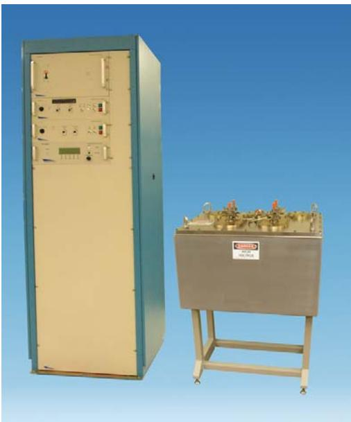
*Figure 5. PEF pilot plant. Capacity up to 400 l/hr. Power electronics in cabinet on left; four-chamber processing unit on right.*
