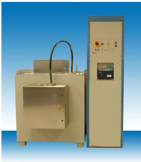
*Figure 1. Commercial PEF System for wastewater treatment. This system is rated at 35 kV, 350 A peak pulses. The modulator is on the left, with the treatment chamber in the 'sidecar' box shown in front. The rack on the right contains the controls and data logging system.*
