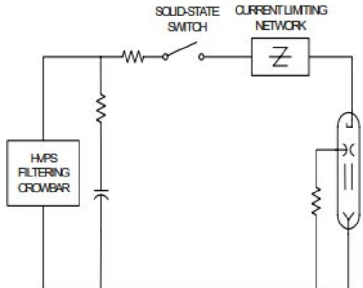
*Figure 1. Schematic showing cathode pulsed VED transmitter with solid-state switch in series between the power supply and VED cathode*
