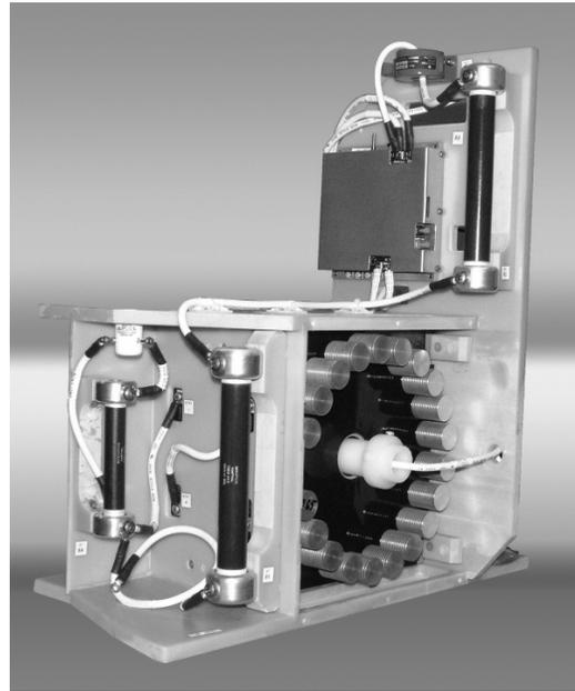
Figure 5. This solid-state cathode modulator assembly replaced the entire AN/SPQ9A mod-anode modulator (HVPS, PFN, SCR switch, pulse transformer, test load), and crowbar circuit.
