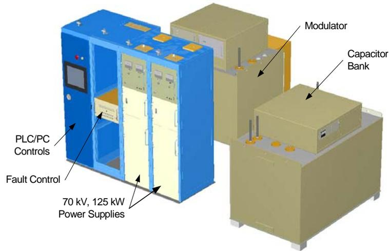
Figure 6. HUSIR transmitter HPA mechanical design. The driver electronics are similar.
