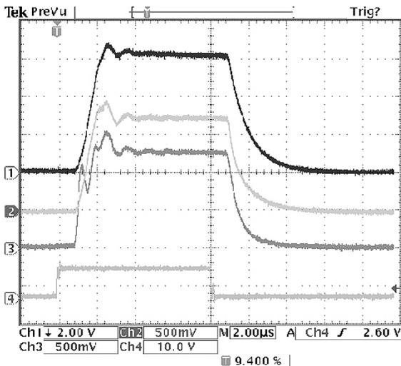
Figure 4. Sondrestrom Modulator Pulse (trace 1 - 130 kV, trace 2 - 120 A). Modulator gate pulse shown in trace 3. Measurements made at the modulator output, and show the cable impedance mismatch. Ringing is not seen on the klystron cathode.
