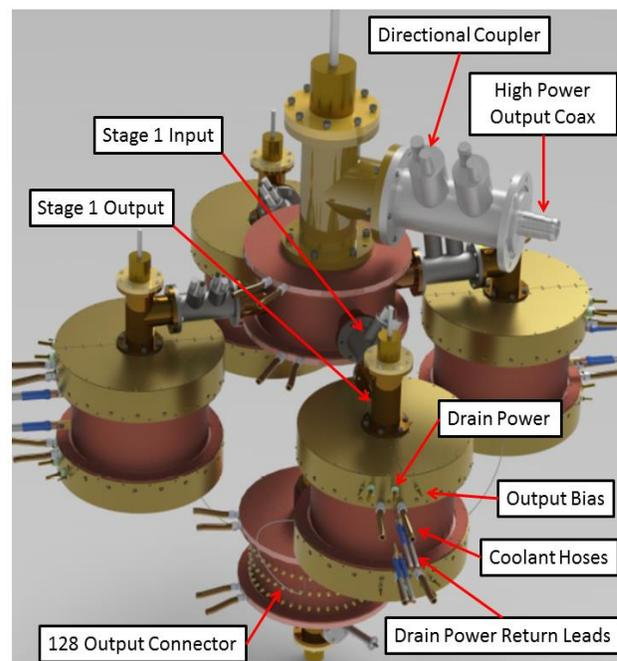
Figure. 3: Arrangement of 200 kW-class transmitter based on four cavity amplifier / combiner modules.
