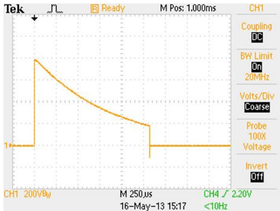
Fig. 3. Pulse voltage without the regulator, 200 V/div, 250 \mu s/div.
