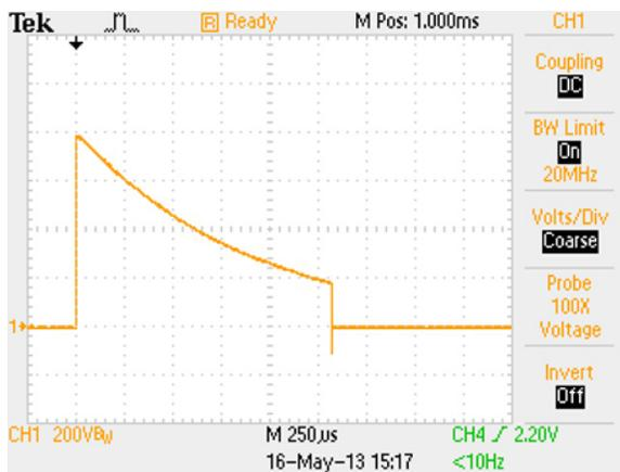
Fig. 3. Pulse voltage without the regulator, 200 V/div, 250  $\mu$ s/div.
