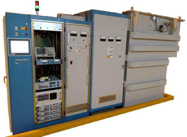
Fig. 1. ESS Klystron Test Stand, showing controls and auxiliary supplies in the left cabinet, the high voltage power supply (center-left), the high voltage modulator cabinets (center-right), and transformer (far right).
