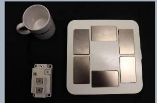
**IGBT used for Pulse Switches (9x9 pkg)** Each IGBT is rated at 5.2 kV, 3 kA peak. 16 of these IGBTs are used in the PGS.
