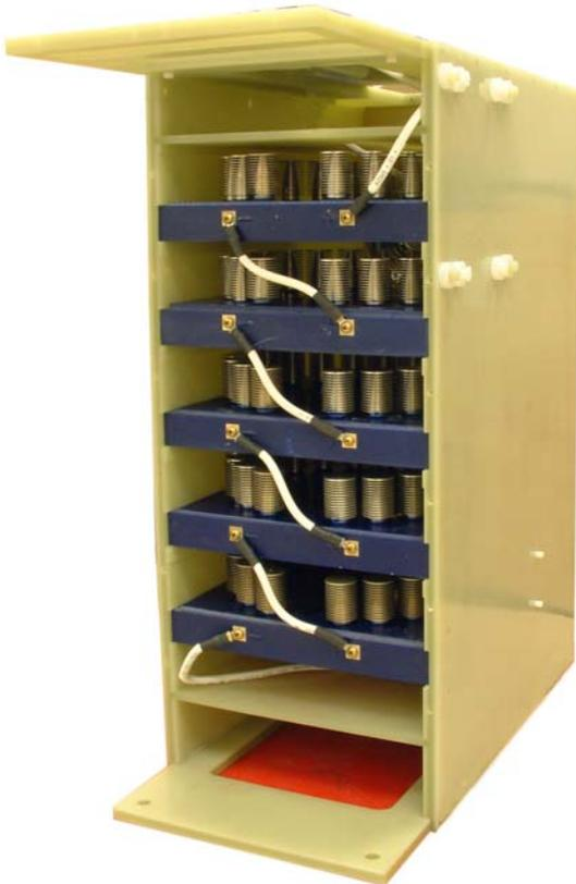
Figure 8. Solid state cathode switch assembly (modulator).
