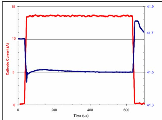
Figure 11. Cathode voltage and current pulse into a single TWT.
