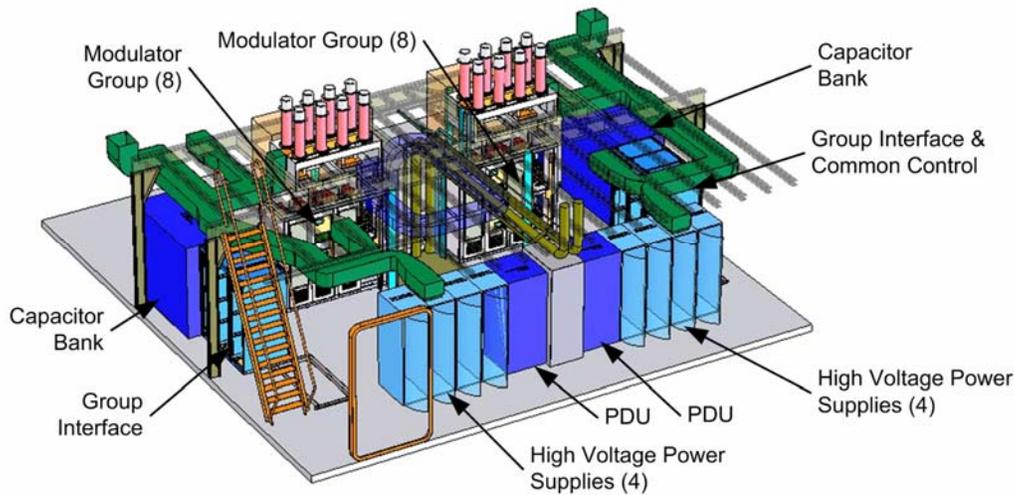
Figure 5. Layout of the new Cobra Judy S-Band radar transmitter. The radar's sixteen TWTs are arranged in two groups of eight, each group having its own electronics. The new electronics for each TWT group consists of one modulator assembly for each of the eight TWTs, two Power Distribution Units (PDU), four (N+1) power supplies, a filter cabinet with a linear voltage regulator, and a capacitor bank.
