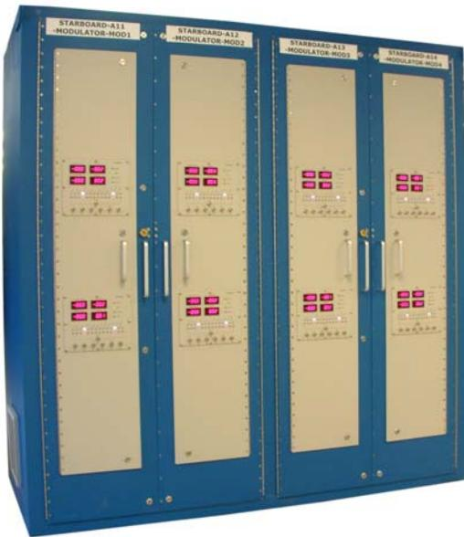
Figure 6 Eight TWT modulator assemblies are located in these cabinets. The eight TWT cathodes will be located directly above this cabinet in the final installation. Each modulator assembly has its own fault control panel as shown in Figure 9.
