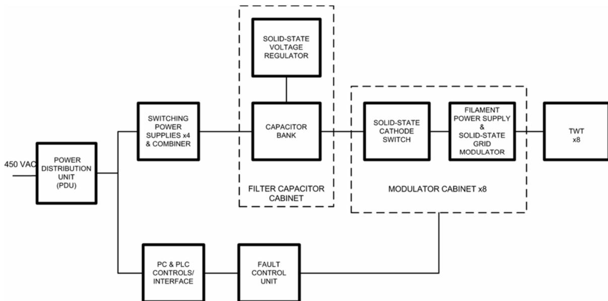
Figure 4. Block diagram of the new CJS transmitter. Diagram represents just one of two identical groups making up the transmitter.
