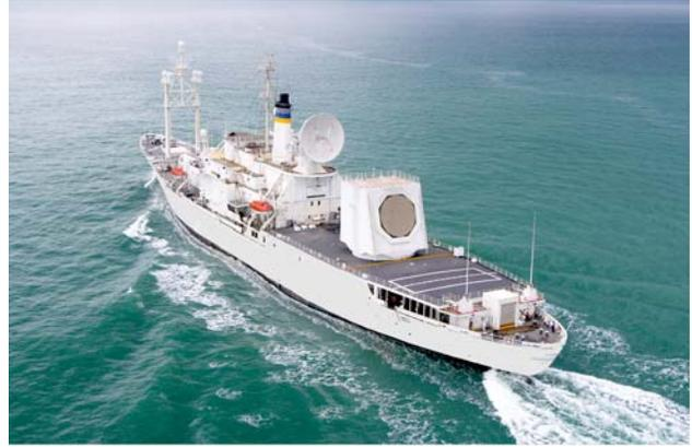
Figure 1. USNS Observation Island. The Cobra Judy S- band radar array is located aft of the Cobra Judy X-band dish.
