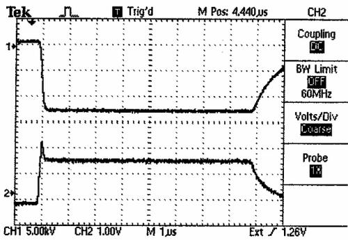
Figure 6: AN/SPG-60 Pulse, 13.5kV, 25 kHz, 8  $\mu$ s
