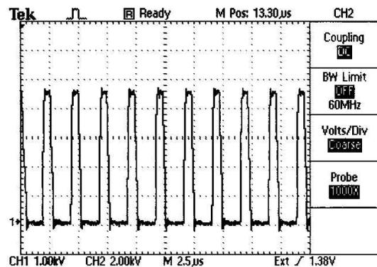
Figure 7: 4.5kV, 400kHz pulse
