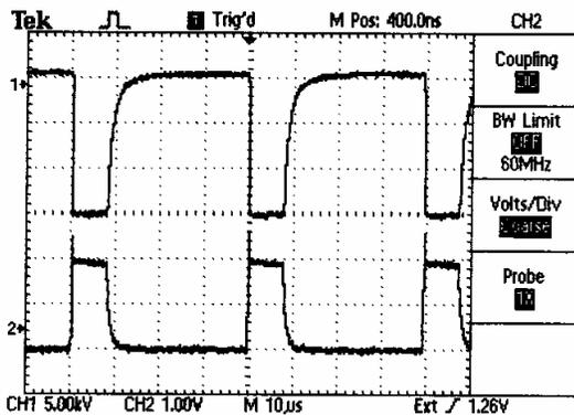
Figure 4: AN/SPG-60 train, 15kV, 25 kHz, 8  $\mu$ s
