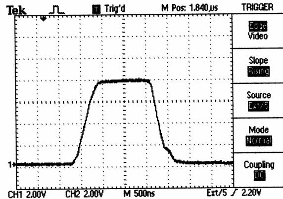
Figure 5: Transmitter pulse 8kV, 100kHz, 1.5  $\mu$ s
