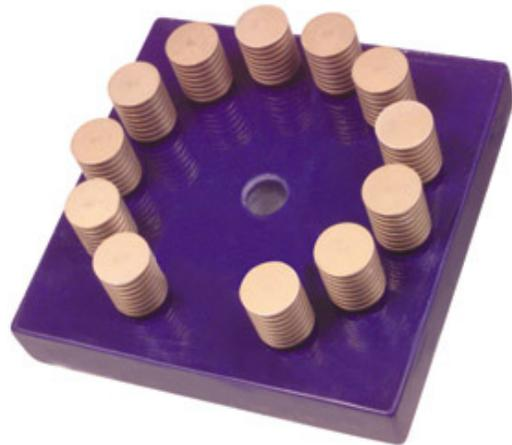
*Figure 1: 9kV, 30A Solid State Switch Module
