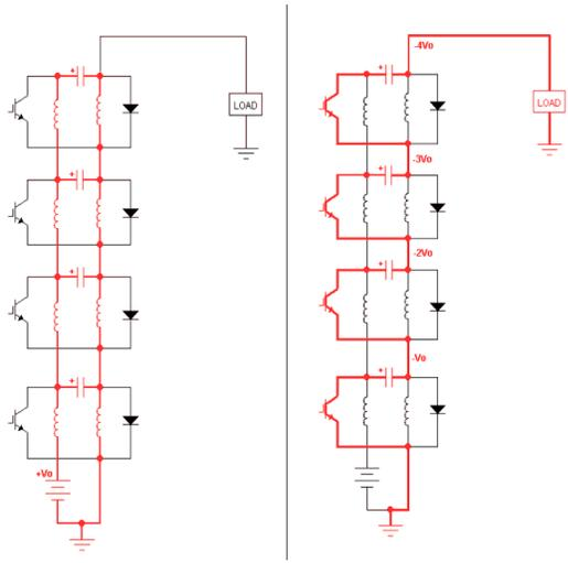
**Figure 2.** Marx bank theory; current flow shown in red. During charging (left), capacitors are charged in parallel at low to medium voltage. During the pulse (right), capacitors are erected in series to achieve high voltage output.
