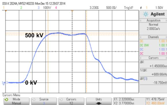
**Figure 3.** Output pulse voltage with 48 plates, showing 500 kV with staggered plate switching to optimize flat top. 106.2 kV/div, 500 ns/div.
