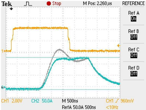
**Figure 4.** Module control tests at 60% full voltage (280 kV, 30 modules at 9.5 kV) into a resistive load. Gray trace is voltage when 30 modules are turned on at once. Green trace is voltage when 21 modules are turned on at once and the remaining 9 modules have delayed turn-on.
