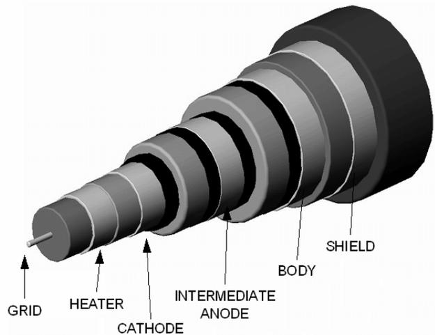
Figure 2. The key elements of the multi-concentric 500 kV cable are two high voltage laminated dielectric gaps (body-IA and IA-cathode), a low dispersion high impedance grid pulse core, and 40A heater-cathode conductors. The entire cable is approximately 3" diameter.
