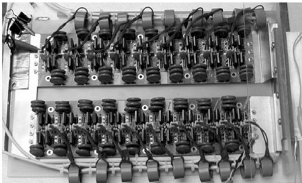
**Figure 5.** A series/parallel array of 1200 V IGBTs in discrete TO-247 packages makes for a very fast hard switch. This assembly is capable of 11 kV operation, with about 25 ns risetime into a 100 Ω load.
