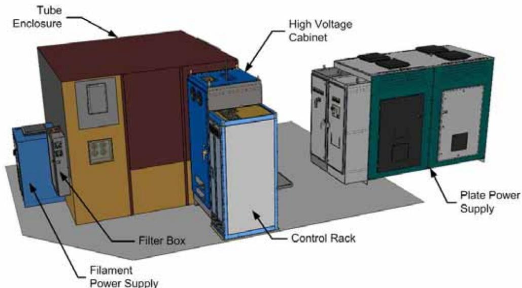
Figure 2. Tetrode test stand assembly.
