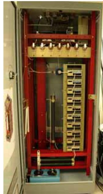
Figure 4. High voltage cabinet interior, showing the solid state switch (R), consisting of ten 3.3 kV switch modules connected in series.
