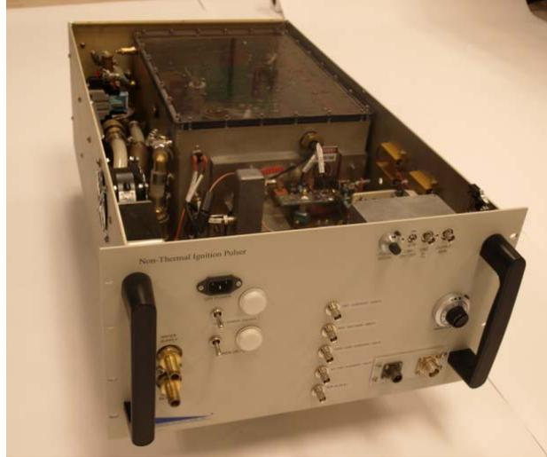
*Figure 1. Fast ignition laboratory pulser delivered to the Air Force Research Laboratory.*
