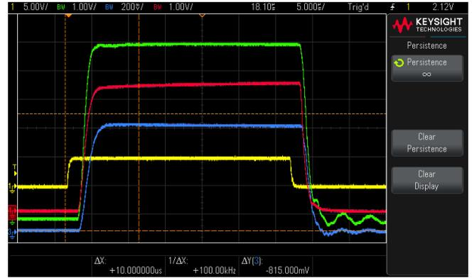
Fig. 2. Cathode Pulse. 30  $\mu$ s pulse, CH1: CMD (Yellow), CH2: Cathode Voltage (Green 20KV/V), CH3: Cathode Current (Blue, 100A/V), CH4: Primary Current (Red, 100A/V).
