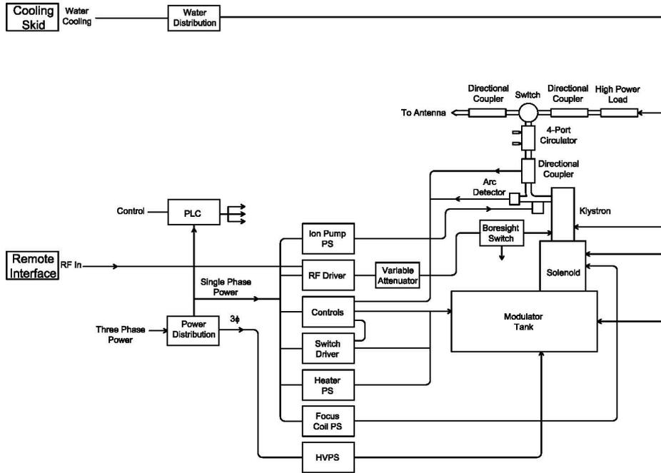
Fig. 3. Simplified Transmitter System Block Diagram.
