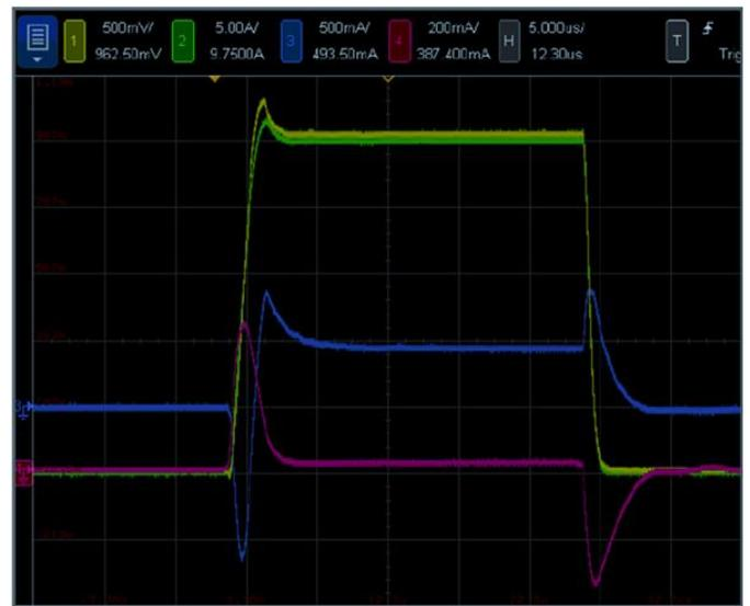
Fig. 3. Typical Waveform at 20 kV Cathode voltage, 100 Hz PRF, and 25  $\mu$ s pulse width (CH1: Cathode Current 10 A/V, CH2: Collector Current 10 A/V, CH3: Body Current 1 A/V, CH4: Mod Anode Current 1 A/V).
