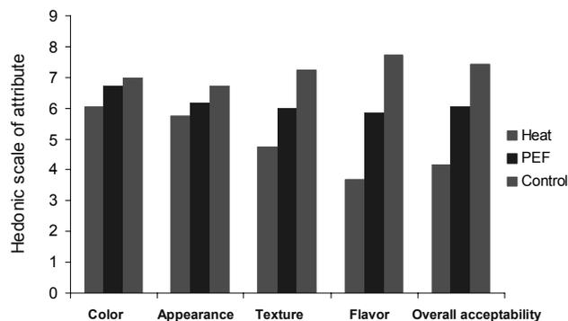
FIGURE 4. PEF results versus pasteurization. Left bar represents heat, middle bar PEF, right bar is control (Source: OSU)
