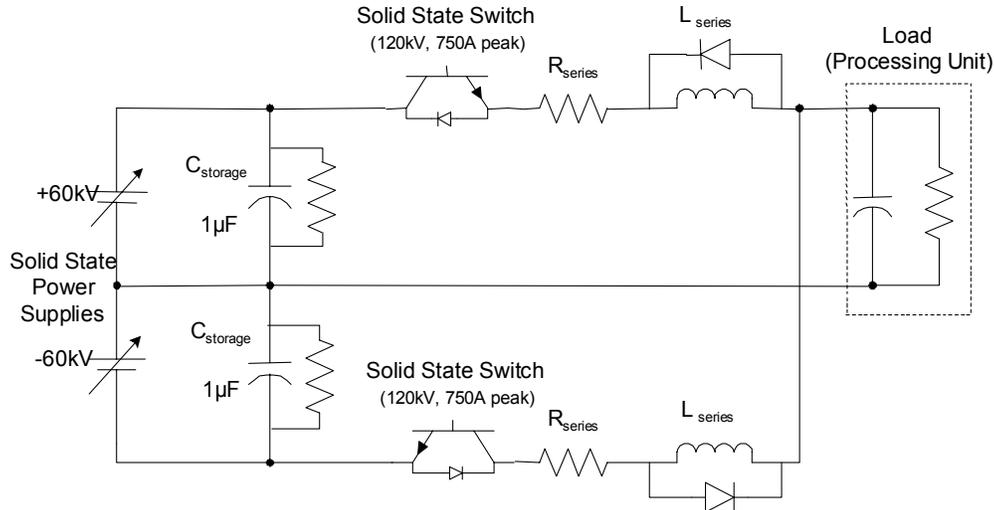
FIGURE 2. Bipolar PEF system block diagram
