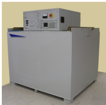
Figure 4. Solid State Modulator tank, with controls located on the lid.
