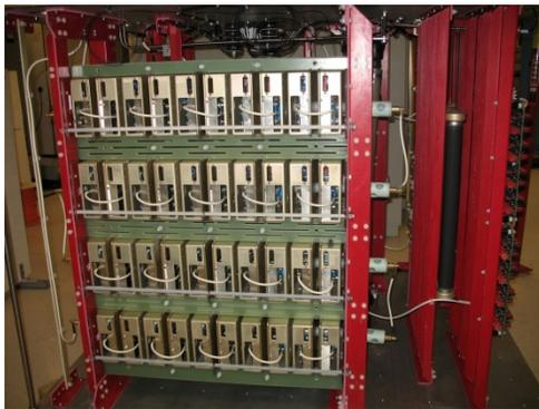
Figure 3. Switch plate array in the transmitter's modulator. The entire assembly is submerged in oil.
