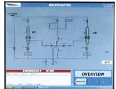
A graphical PLC control system provides state control and fault reporting for the entire transmitter.
