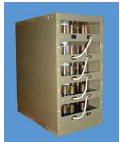
This 45 kV, 50 A solid-state opening switch replaced the vacuum tube crowbar on the Invincible's GrayStar X-band radar.
