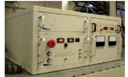
The test stand's modulator controls include fast fault detection and first fault identification.
