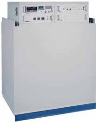
PowerMod 100-150 solid-state modulator, 100 kV, 100 A. Size 50" w x 36" d x 64" h. Oil and water cooled.
