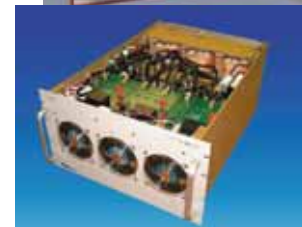
Modular DC-DC Power Converter. In this configuration, each drawer is rated to 30 kW, with the cabinet rated up to 150 kW total, with N+1 redundancy.
