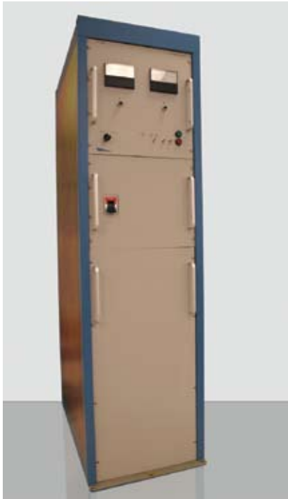
Free-standing 50 kV, 150 kW switching power supply. Enclosure is 24" w x 36" d x 60" high.
