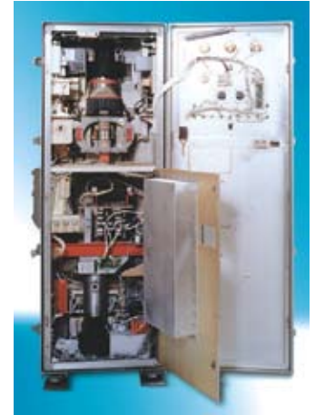
AN/SPG-60 radar transmitter enclosure with DTI modulator retrofitted in lower compartment.
