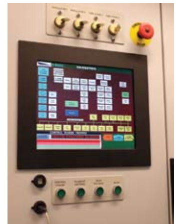
A programmable logic controller (PLC) is featured on some DTI' transmitters for enhanced operator control, fault handling and diagnostic capabilities. The operator controls the transmitter via this flat-panel touch screen and graphical user interface.
