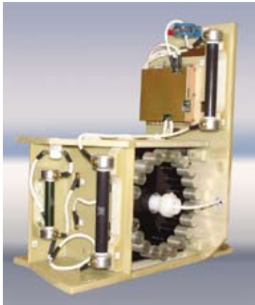
This solid-state cathode modulator assembly replaced the entire mod-anode modulator and crowbar circuit for the AN/SPQ-9A radar.
