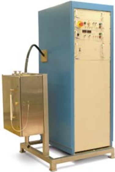
25 kW PEF treatment system. The enclosure containing the PEF treatment chamber is shown on the left. The tall cabinet contains the pulse modulator, controls, and high voltage power supply.
